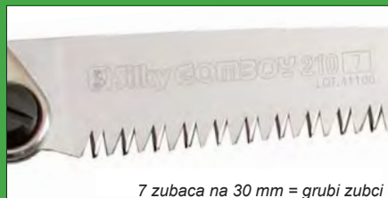
7 zubaca na 30 mm = grubi zubi
